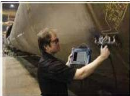
Pipeline Thickness Gauging
